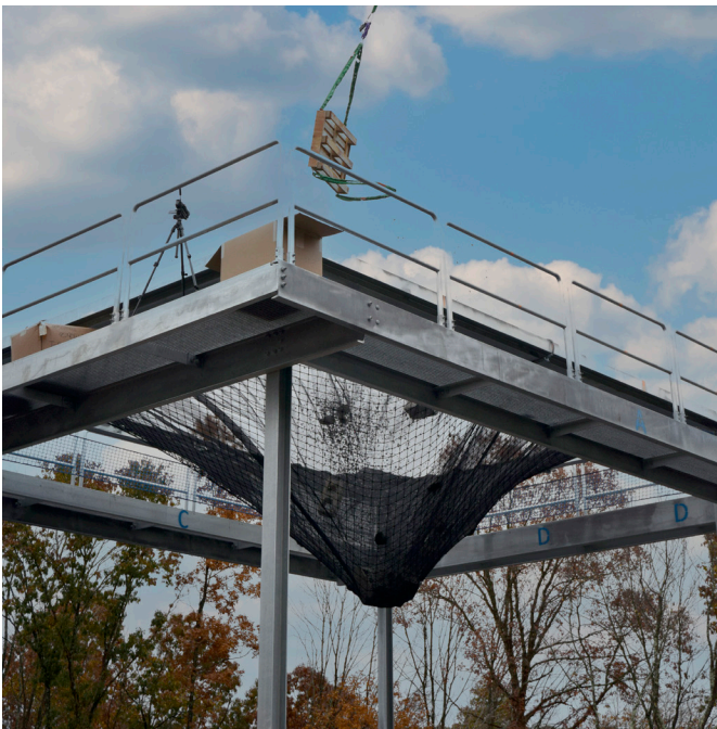
Dynamic PSN testing at InCord's on-site test frame.
